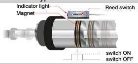
When the piston's magnet approaches the magnetic sensor, the internal reed switch will detect the change of magnetic field and close the contacts.
