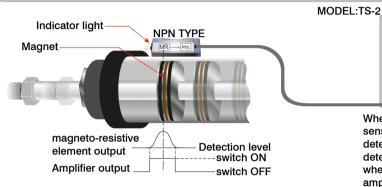
When the piston's magnet approaches the magnetic sensor, the internal magnetouresistive element can detect the internal magneto-resistive element can detect the change. Switching output is achieved when this signal is amplified by the operation amplifier circuit in the magnetic sensor.
